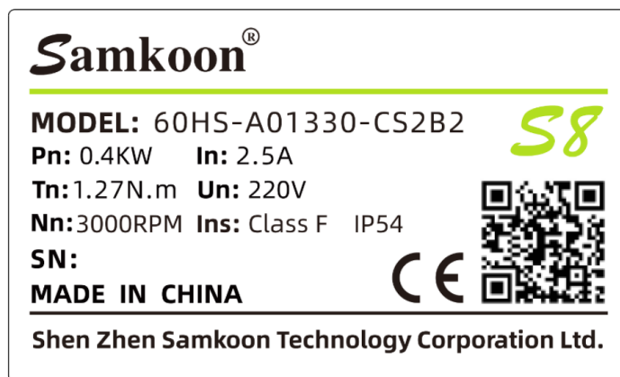
Figure 2-6 Motor Nameplate Identification
