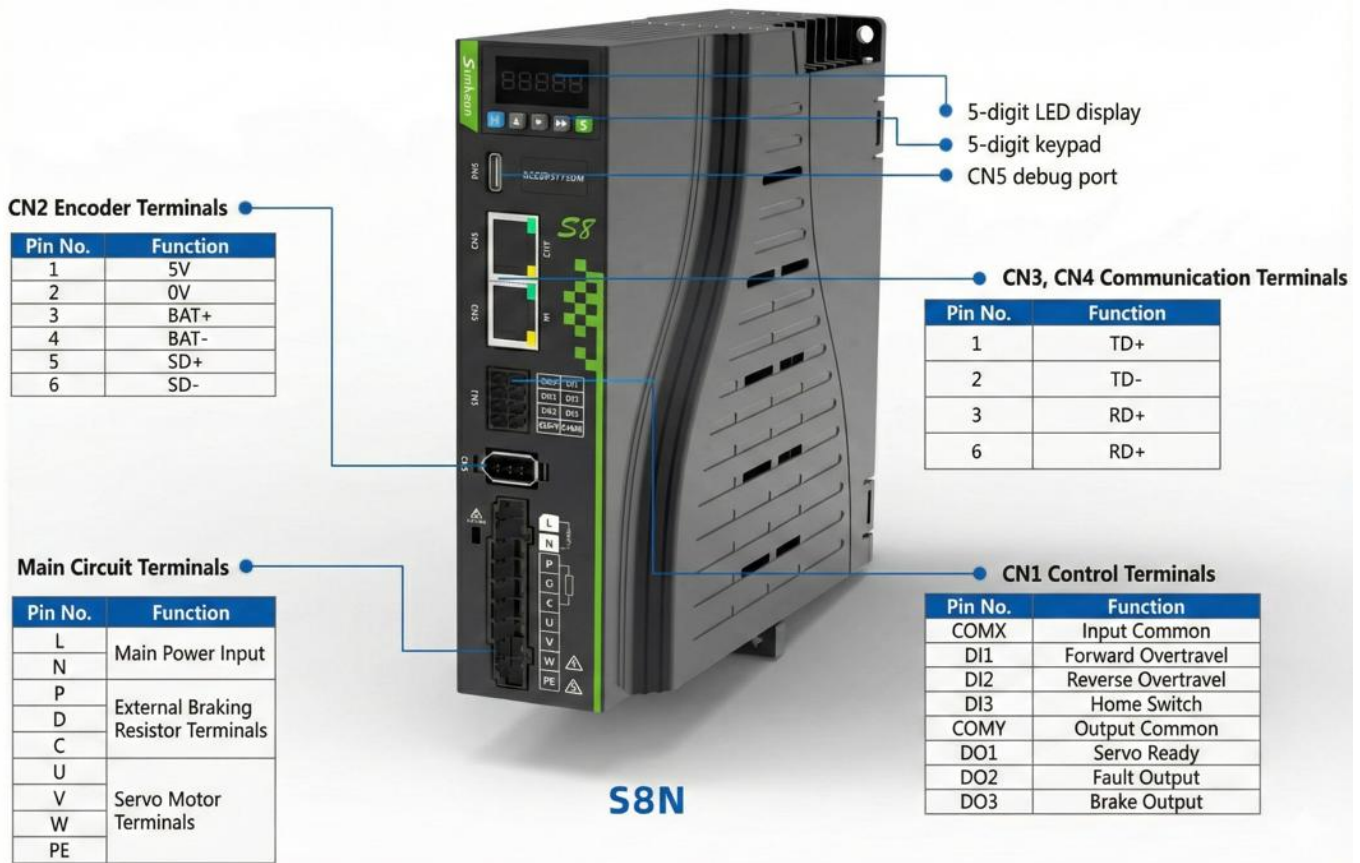
Figure 2-3 Composition Structure of S8 Series Servo
